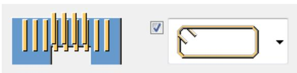
Stirrups are created instead of U bars when the distance between the edges in the panel or the slab is so small that the U bars do not get the required cover thickness.
