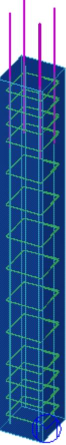
A 3D perspective view of a vertical concrete column. The column is shown in a light blue color. A network of yellow and red lines represents the reinforcement cage, consisting of longitudinal bars and horizontal ties. The cage is shown in a cutaway view to reveal its internal structure. | Rebars in a concrete column. |
