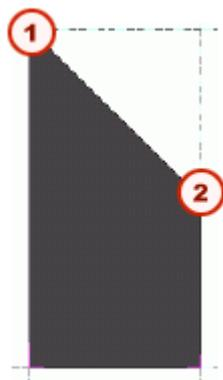
The diagram shows a dark gray contour plate with a slanted top edge. Two points are marked with red circles and numbers: '1' at the top-left corner and '2' at the top-right corner. Dashed lines indicate the bounding box of the plate. | <p>Контурная пластина на виде модели.</p> <ol style="list-style-type: none"><li>1. Первая точка создания</li><li>2. Вторая точка создания</li></ol> |
